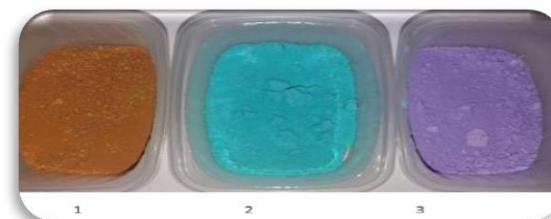
Organic metal salts of variable valence: 1 – iron carboxylate; 2 – copper carboxylate; 3 – cobalt carboxylate
