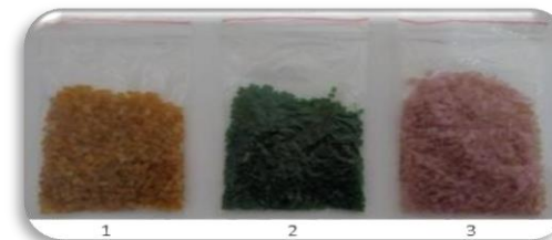
Multifunctional concentrate additives based on: 1 – iron carboxylate; 2 – copper carboxylate; 3 – cobalt carboxylate
