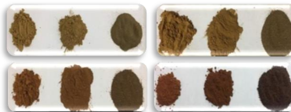
Fractional glauconite pigment can be thermally activated at various temperatures
