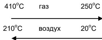
$$\Delta t_{\bar{o}} = 250 - 20 = 230^{\circ}\text{C}$$
